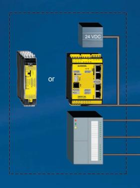
■ The new safe input expander module SRB-E-PE can have not only electromechanical safety switches with dry contact outputs connected to it but also electronic safety sensors with OSSD outputs. For larger systems, the input expander SRB-E-PE can be connected in series.
