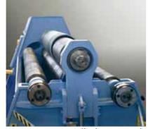
This allows to get parts rolled to a much tighter diameter (down to even less than 1.1 times the top roll diameter), a 30% benefit in tighter diameters on the Davi Pivoting Swing Guides, vs. the old rectilinear guides.
