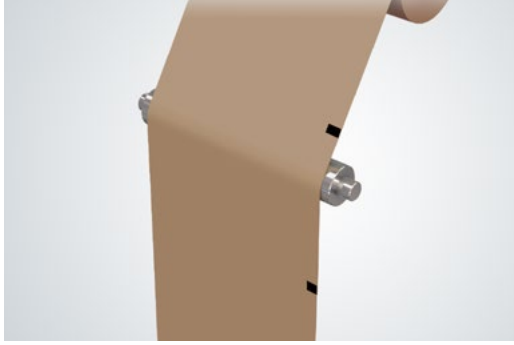
Registration mark detection on film
