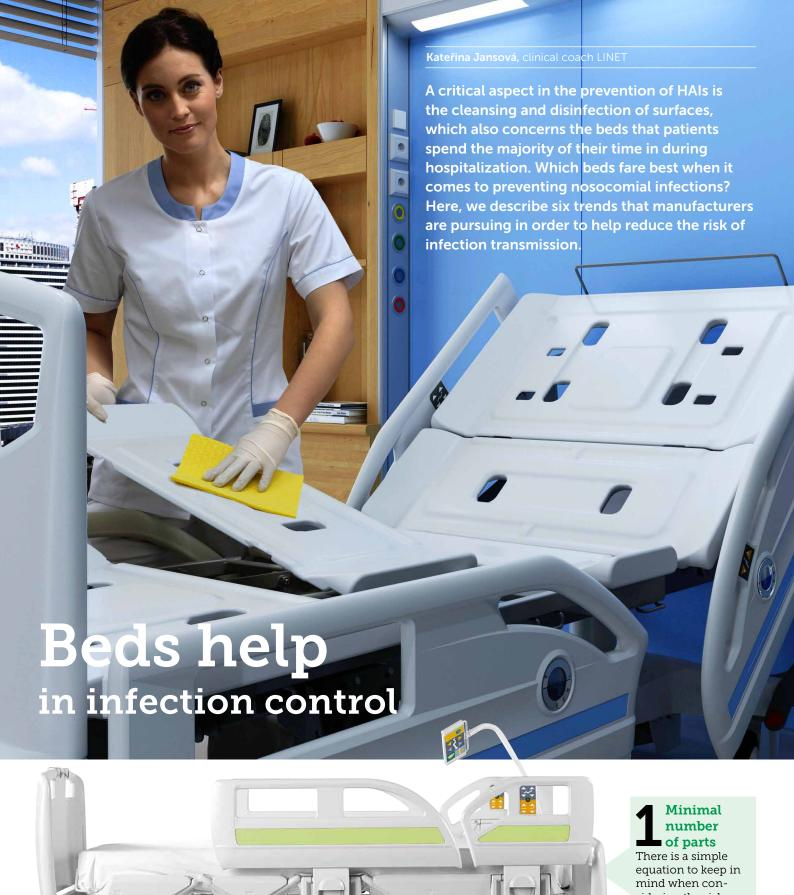
There is a simple equation to keep in mind when considering the risk of contamination: More parts mean more places for contaminants to take hold and more complicated cleaning too. Therefore, the components in modern beds feature designs that are smooth and require very few joints and small parts.
