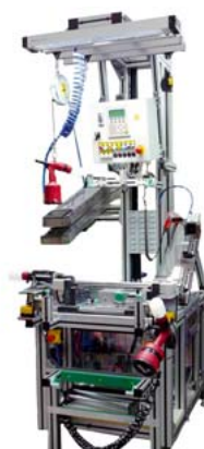
Riveting workstation with TIOS control
