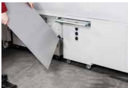
Release the chippings container
