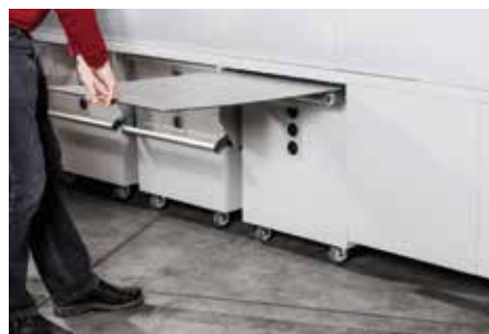
Push in the dust compartment
