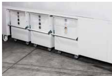
Clamp the chippings container into place
