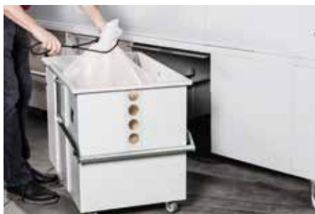
Replace the chippings container
