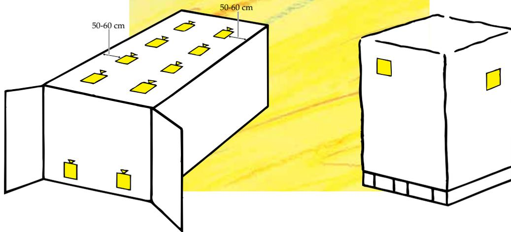
DRY-BAG® s should be placed evenly on top of the cargo, with one or two at the bottom near the doors.
