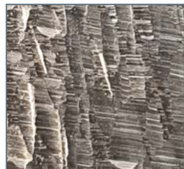
A-0006 Surface. Average 44 \mu\text{m}
