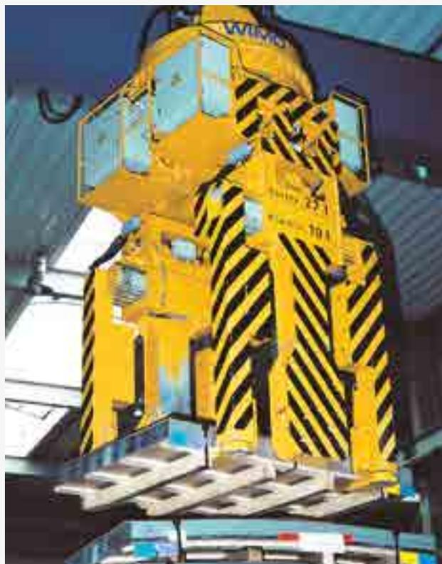
Multi-purpose tong with horizontal rotary drive system
