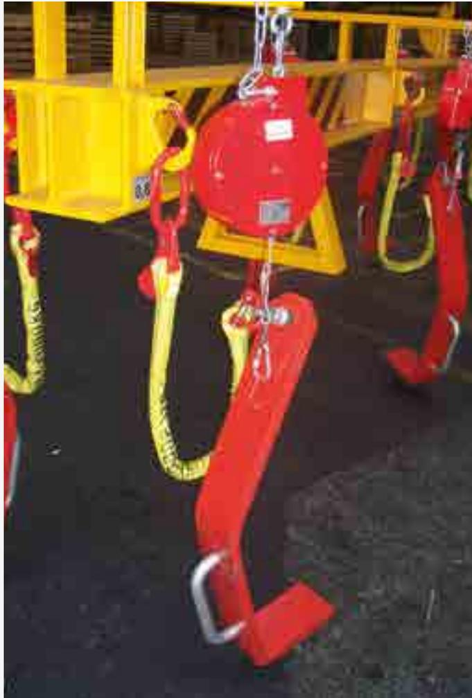
Spreader with plate hooks suspended on spring balancers which can easily be attached to the sheet metal stack and remain stuck
