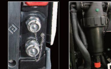
Water filling filter + Storz DN 25 water coupling
