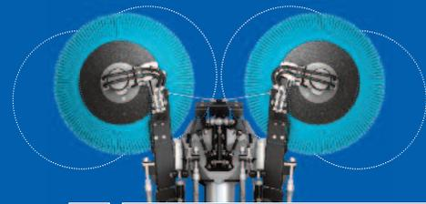
The Mathieu MC110 sweeper offers many attributes. Nimble and compact, it can negotiate narrow streets with great agility. Articulated and with a tiny 1.80 m approx. turning radius, it can virtually turn on the spot. And with a height of less than 2 m, it's the ideal sweeper for underground car parks. Its two-brush pushed sweeping system with wide side and front swing gives it even greater agility for cleaning 90° corners and around urban amenities.
