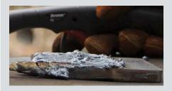
When using FlushCut consumables, operators can expect to leave less than 5 mm of material on the workpiece after the removal of a lug, attachment or pad eye.
