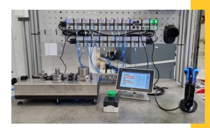
Imposing air and probe control station for rapid inspection of a multitude of characteristics on 25 connecting rod models.
