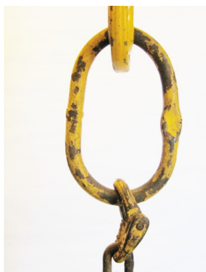
Ovalring Deformation, overbelastning
