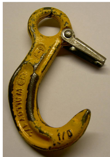
Krog Deformation, overbelastning
