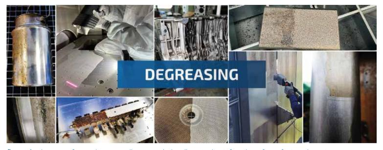
**Degreasing:** lasers are often used to remove oil, grease and other oily contaminants from the surfaces of automotive parts, machine components and tools. This prepares parts for further processing such as welding, painting or bonding.
