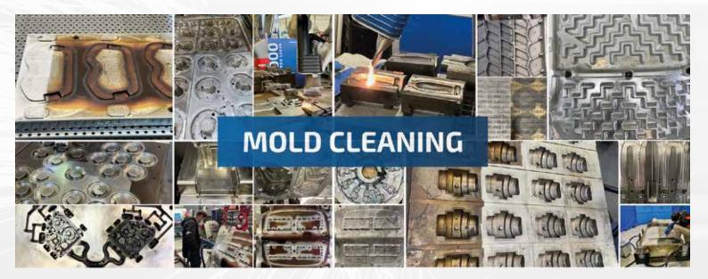
Mold cleaning: in the plastics, rubber and metalworking industries, lasers are popular for cleaning molds of deposits and material residues without disassembly. This minimizes downtime and increases production efficiency.
