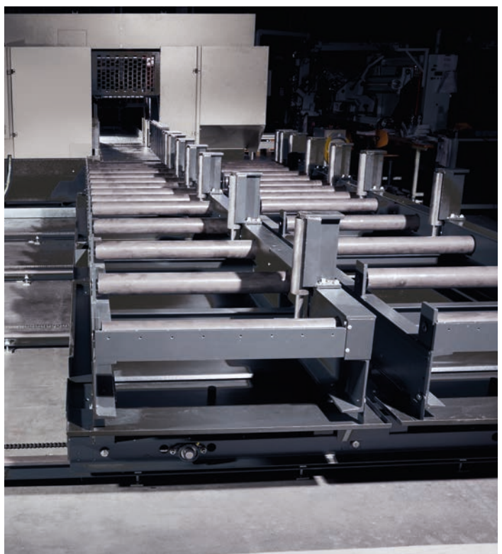
Double roller conveyor for automatic change of material (win 3.3, 4.6, 5.6 and win tube 5.0)
