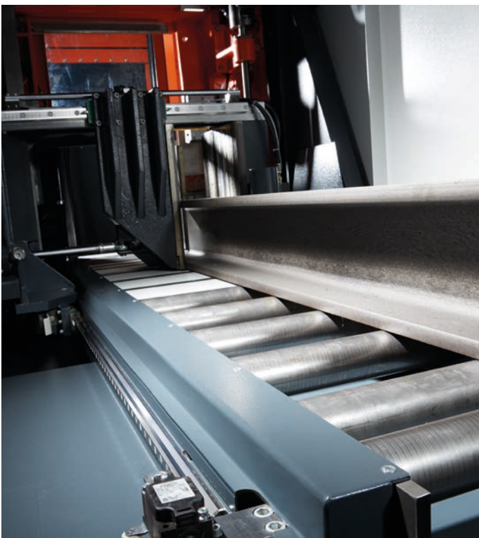
Material feed with 1500 mm feed length (3.3, 4.6 and 5.6)
