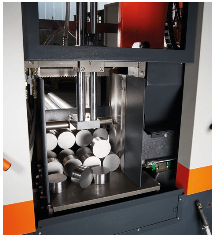
Hydraulic bundle clamping device incl. opening and closing limit
