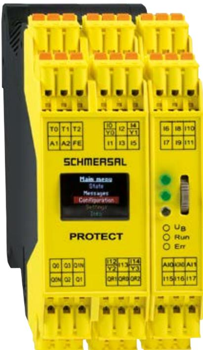
Four different programs are available. Each program can be precisely adapted – without any programming knowledge, simply with the menu and clear text messages – to the specific application case. The drop-out delay and the debounce times can be set individually, and numerous parameters such as the short-circuit monitoring can be set as required – a definite advantage in comparison with safety relay modules.
