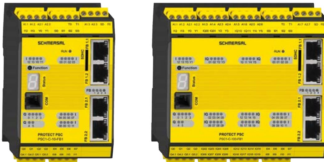
The safety control system PSC1 consists of freely programmable compact safety controllers with I/O extension modules for signal processing of EMERGENCY STOP switches, guard door switches, light grids and other mechanical and electronic safety switchgear. Additionally there is the possibility via numerous functions to monitor axes. Using the universal communications interface, a connection can be established to all the standard field bus systems.
