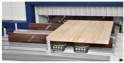
Easy positioning of heavy work pieces and large panels with the lifting support.
