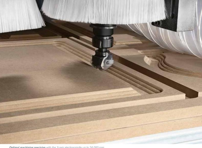
**Optimal machining precision** with the 3-axis electrospindle up to 24.000 rpm.
