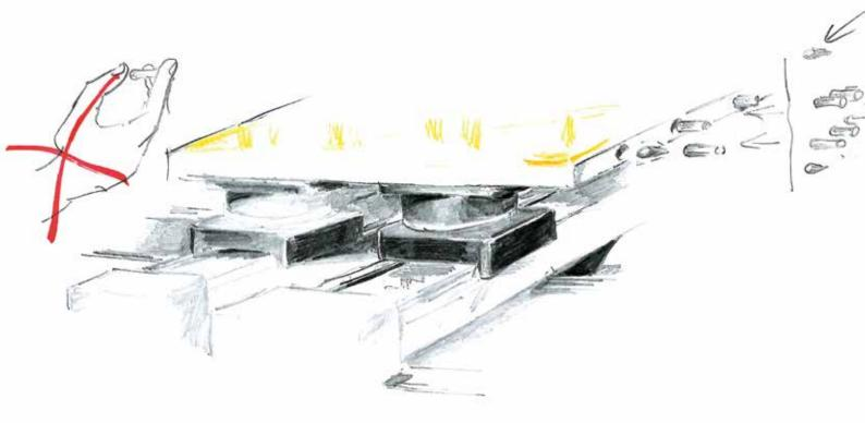
Optimisation of productivity with no more time wasting for cleaning operations, thanks to the use of glue capsules, contrary to traditional dowelling devices where it is necessary to remove the remaining drying glue from the various components after a temporary production-stop.
