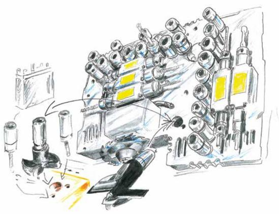
HINGE DRILLING: ONE STEP WORTH THREE! Possibility to carry out 3 simultaneous drillings with a single head integrated in the main drilling unit.
