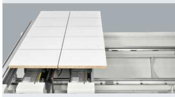
No problem for the sliding of vacuum pods or clamps thanks to the blowers positioned along the whole rail that guarantee a constant cleaning.
