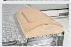
Easy and quick positioning of locking accessories such as MPS vacuum pods and the practical MODULSET system with the surface channels structure.
