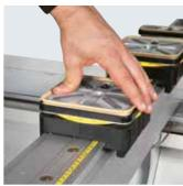
It is possible to add or remove vacuum pods or clamps with a simple movement of the hand; the number and the position are automatically detected.
