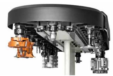
Wide range of tools available to the operator with the rear tool changers up to 32 positions.
