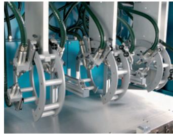
Construction for environmentally friendly lacquering of wiper blades with water based lubricant.
