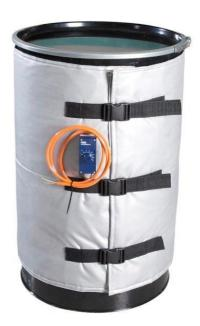
The heating element of the Drum Heaters is stiched into an insulated jacket made from a water resistant, nylon and silicone coated material. Comes complete with quick release buckles for ease of installation and removal. The heating element is shielded with a tinned copper earth braid for safety. All our Drum Heaters are supplied with 3 metres of braided power cable and fitted with a 0 to + 200° C capillary thermostat and 230 volts AC.
