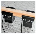
Locking systems It is possible to use clamps or suctions cups to lock work pieces of particular shapes and dimensions.
