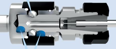
Optimised spring and dampening compensation (+/- 0.5mm)
