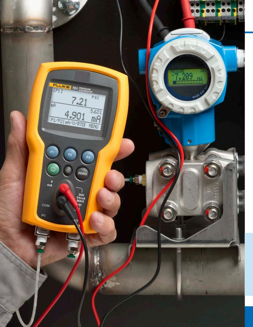
Portable/handheld pressure calibrators
