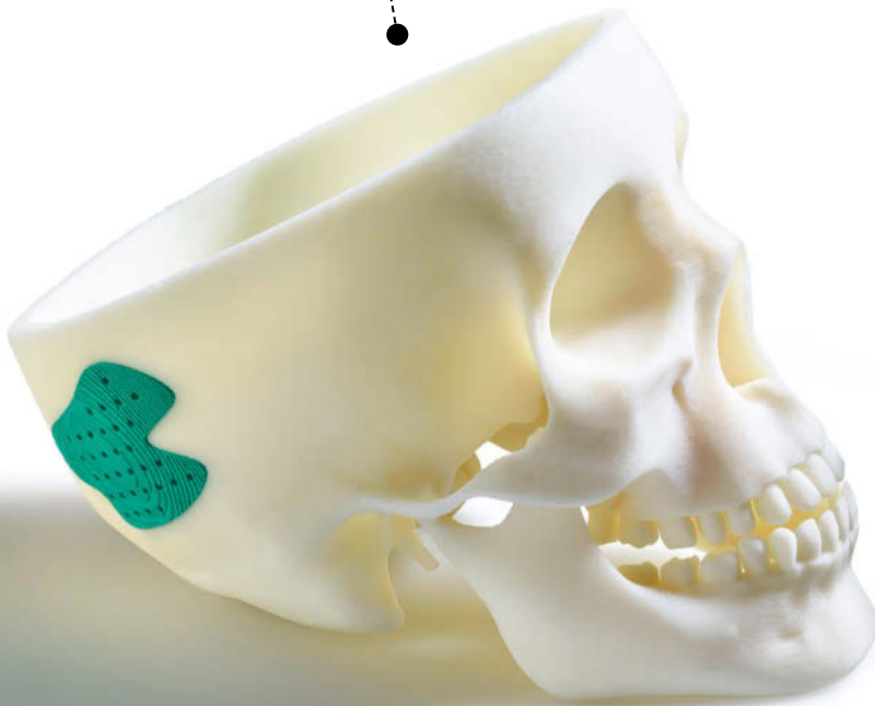
Medical implants: cranial implant made from resorbable polylactide (PLLA).
