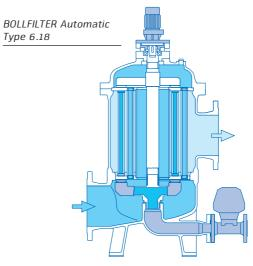
The main field of application for this BOLLFILTER Automatic is water filtration. The internal components are therefore always made of stainless steel. The fully automatic backflushing of the filter element is very efficient. Axial- and cross-flow backflushing is generated with filter candles open at both ends - the bipolar functional principle.
