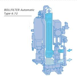
The BOLLFILTER Automatic Type 6.72 was specially developed for smaller flow rates of fuels and lubricating oils. Its special design allows filtration grades up to 6  $\mu$ m. A bypass filter with change-over valve can be integrated to use Type 6.72 as a fuel filter.
