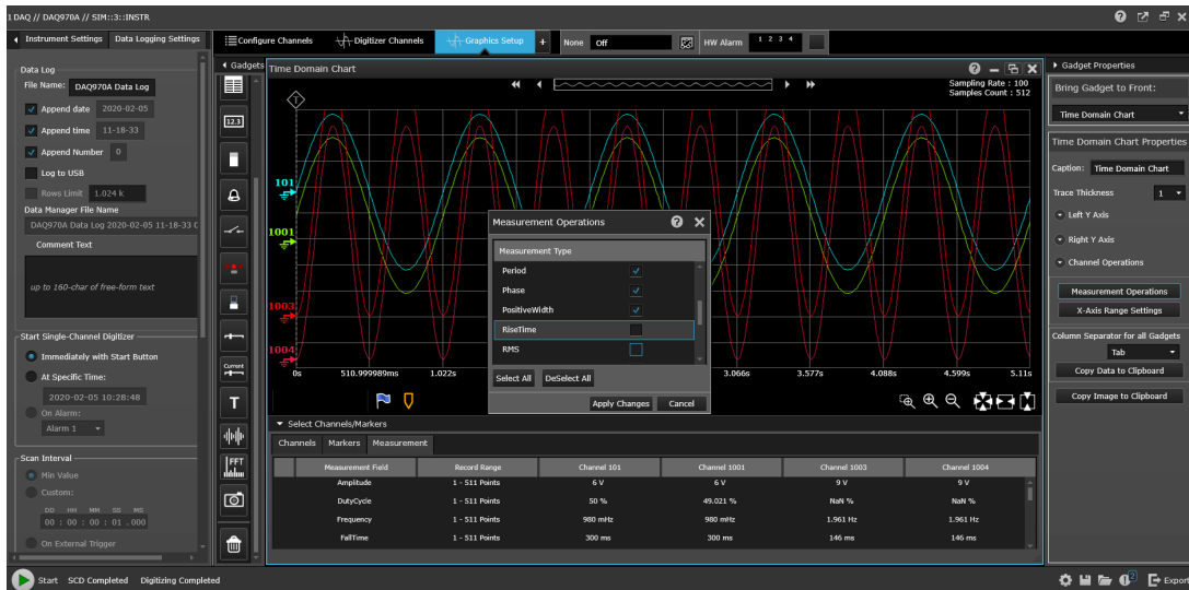
Figure 11. PC DAQ application software that helps display a time domain chart and derives a host of statistical measurements
