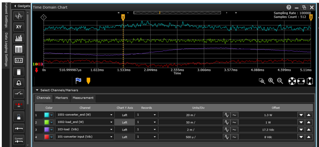
Figure 7. Simultaneous display of source and load power of a DC-to-DC converter
