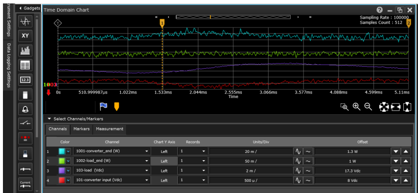
Figure 3. Multiple dynamic signals captured or monitored by a DAQ system
