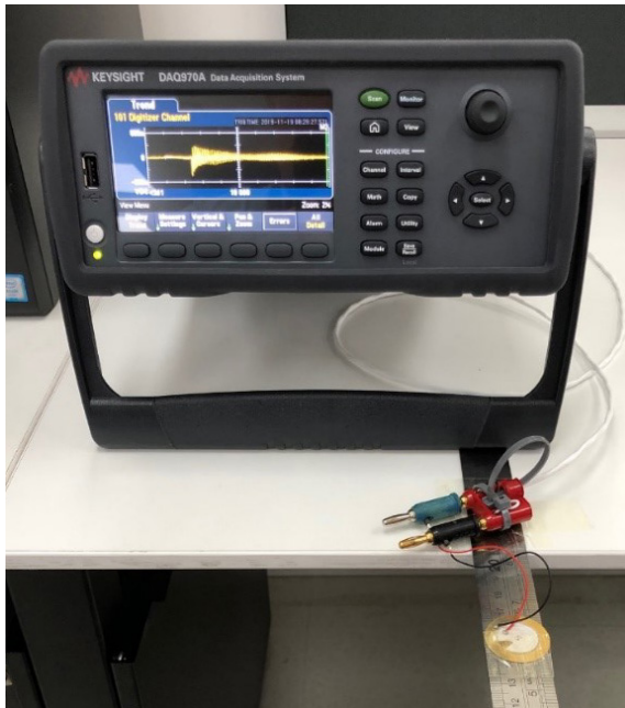
Figure 8. A dynamic DAQ system capturing a cantilever vibration from a piezoelectric sensor
