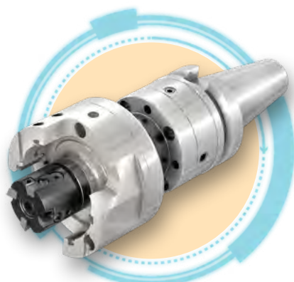
Combined tool for external reaming with adjustable PCD blade and guiding pads and interchangeable head for milling with PCD brazed cartridges
