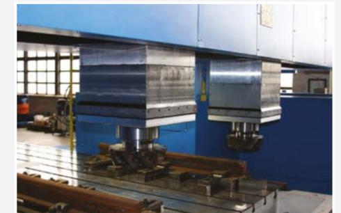
CNC DREH- BOHRMASCHINE
