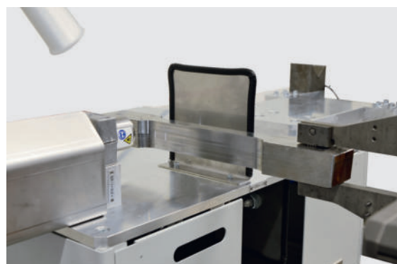
Specimen marking in the automated test centre
