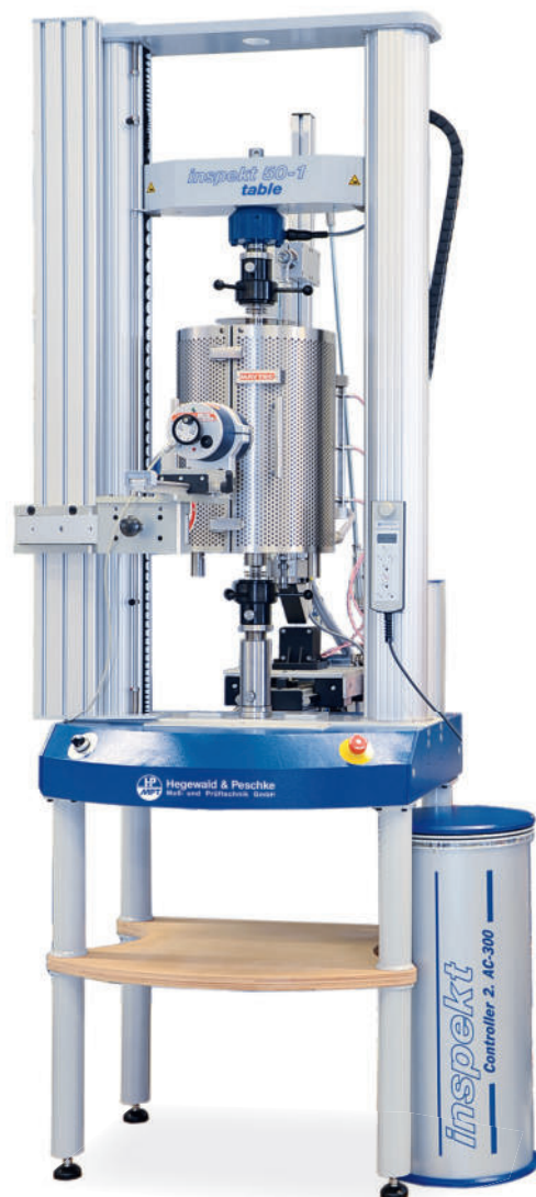
Universal testing machine Inspekt 250 with high-temperature furnace, temperature chamber and additional test room at the side
