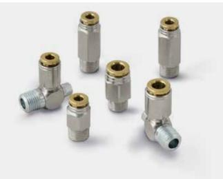
The High Pressure brass push-in fittings series can be used with oils and greases in lubrication and greasing systems, with a maximum pressure of 250 bar thanks to a special crimping gripper. They are available with different threads UNI ISO 7/1 UNI ISO 228/1 and are suitable for rigid and semi-rigid hoses commonly used in lubrication.
