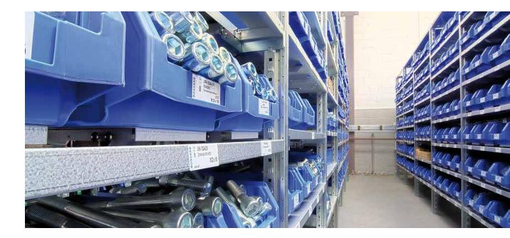
This unique, fully automated system with sensor monitoring is ideal for supermarket areas and line assembly. SmartBin manages anything from small parts weighing just a few grams to large parts of up to 1,000 kg per palette. Weight sensors ensure continuous online inventory monitoring. Orders are triggered automatically and enable a seamless supply.
