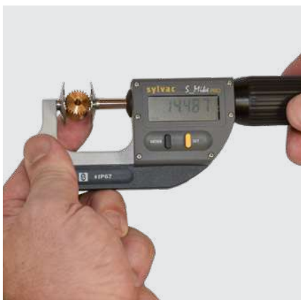
Part measurement with a S_Mike PRO Disk
