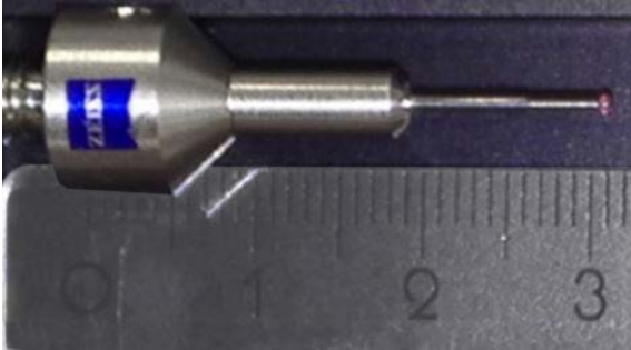
View of the stylus with material build-up in original size.
