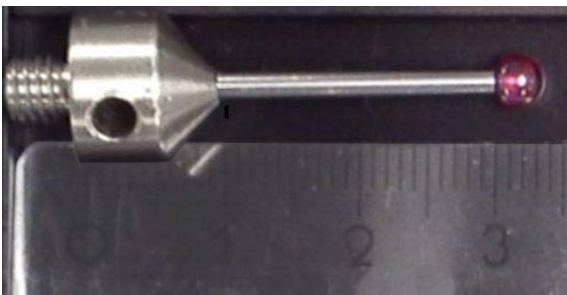
View of the defective stylus in original size.
