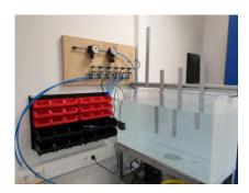
The samples are immersed in a bath of water and the interior of the configuration is air pressurized to a pressure of 0.5 bar for a period of 24 hours.
