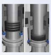
Automatic spindle clamping system
