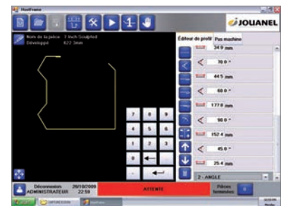
Drawing of a profile directly on the screen
