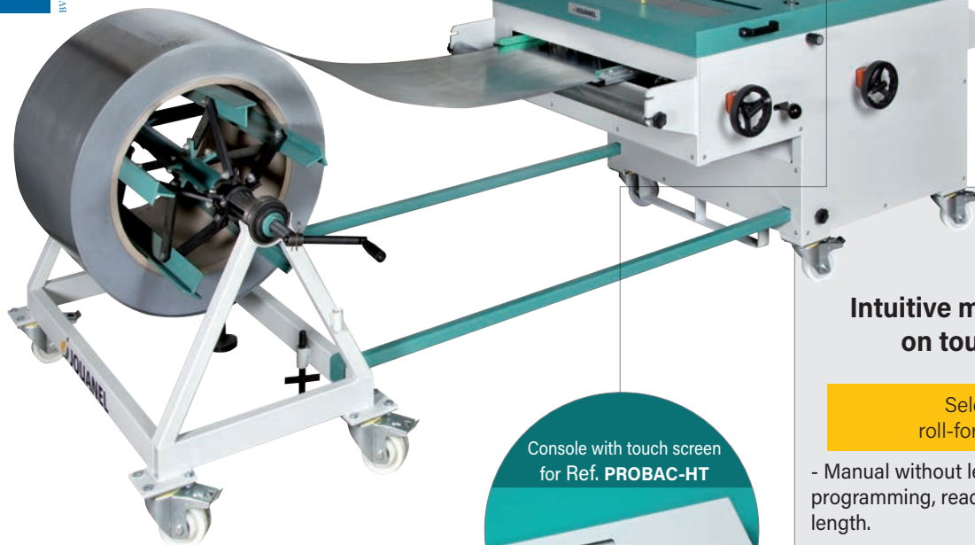
Ref. PROBAC-HT shown with Connecting rails (option) Ref. PROBAC-DVS shown with decoiler Ref. DVS1000
