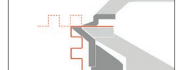
Folding beam with clearance for PTS: PTSL-TDI
