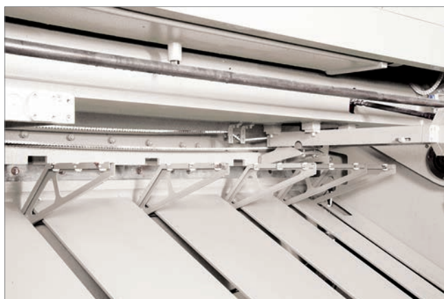
7 Pneumatic sheet holding plate
