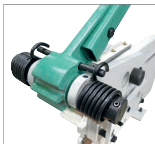
Safety: return spring on the upper blade
