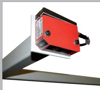
Laser control of the loop
