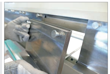
1 Quick disassembly of the segments with pull-device
