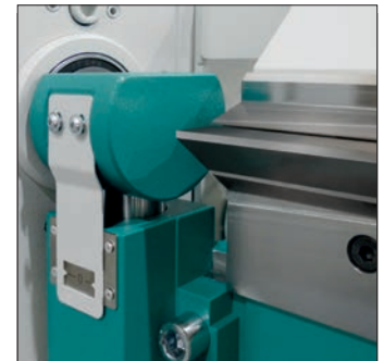
Folding beam with clearance for PTS: PTSL-TDI
