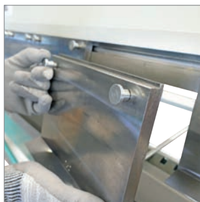
1 Quick disassembly of the segments with pull-device
