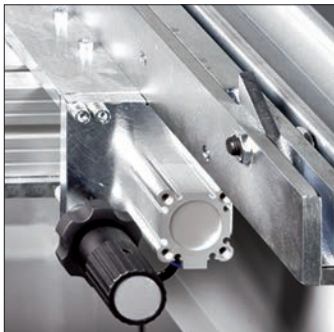
Pneumatic conical folding, manual adjustment
