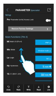
Scroll vertically to find the desired parameter, for example NO/NC configuration (LO Logic)
