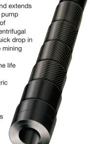
A large copper and gold mining company in Arizona needed to replace hard chrome iron centrifugal pumps on a difficult tailings slurry application. The centrifugal pump impellers were wearing out every two weeks, causing significant downtime and costly repairs. The mine considered several different pump technologies, selecting Watson-Marlow Bredel SPX100 hose pumps. The hose pumps transfer the tailings slurry 2,200 feet away to a separate
