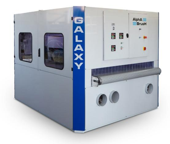
The machine can be supplied with many different types of abrasive or polishing material all depending on application. The spindles are mounted with a bearing plate on the end for extra spindle support. The four sanding units each turn around it's own axis, while the main carousel is also turning.
