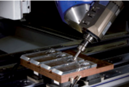
High-gloss trimming of acrylic parts
