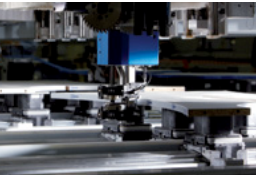
Perfect edge finish with traced combination flush trimming / scraping unit
