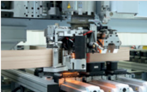
Edge banding for components up to 100mm in height
