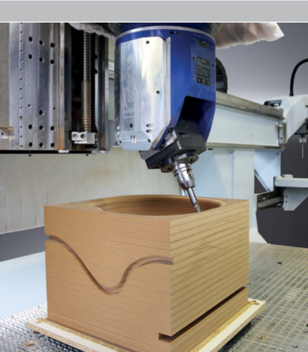
Trimming of components with large Z height
