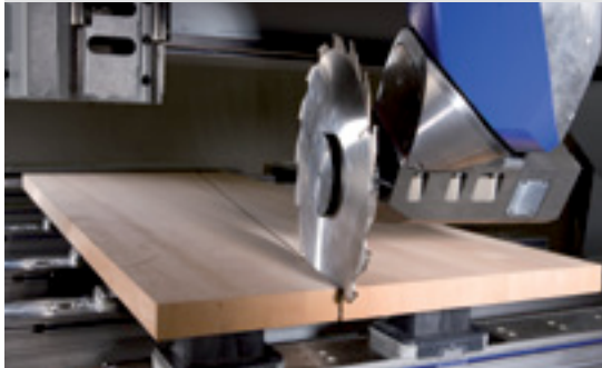
Dividing cuts up to 110 mm in height
