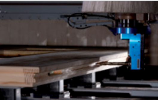
Lock case trimming on front doors
