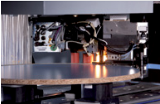
360° edge banding with the powerEdge edge banding unit
