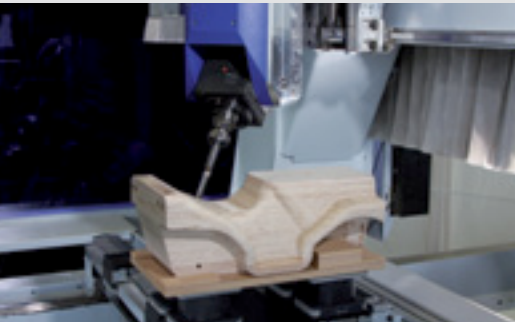
Interpolating processing of freeform components
