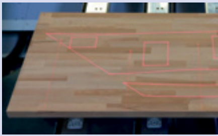
Laser projection of the clamps and the workpiece contour for optimum utilization and simple positioning of raw parts which cannot be aligned at the stops.
