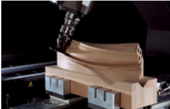
Routing of a stair hand rail
