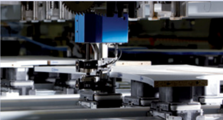
Perfect edge finish due to traced combination flush trimming / scraping unit – efficient processing without tool change.
