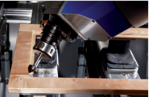
Square corner routing for a glass rebate
