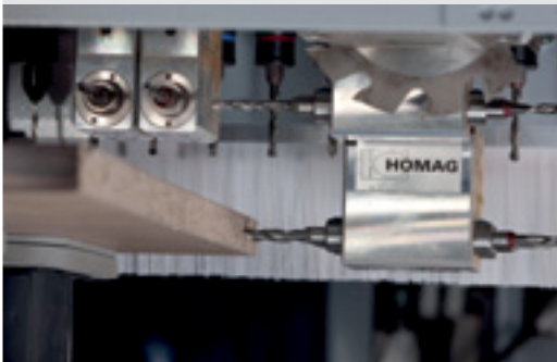
Horizontal boreholes for carcass connections
