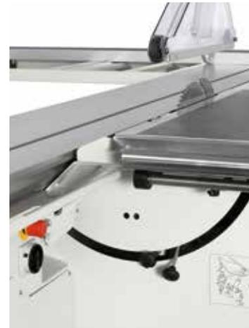
The scoring blade is adjustable from the outside without tools and allows fast and accurate positioning with no play.
