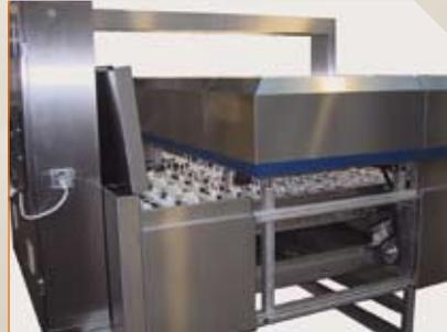
*Even the electrical cabinet of the packer lanes is placed above the egg flow. By simple command, packer lanes can be reprogrammed without stopping the rest of the machine*
