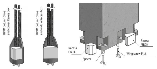
To ensure higher values of concrete cover thicknesses of main anchor bars, in accordance with chapter 1.2.3 of the technical manual, follow these instructions for increased values  $\Delta_c$  of concrete cover:
