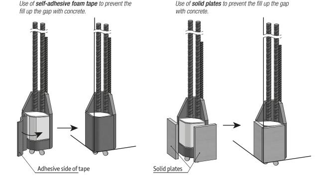
Ensure of thicker concrete cover by self-adhesive foam tape or solid plates
