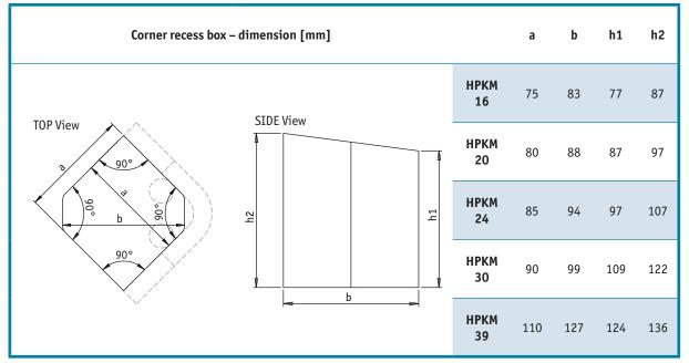
Table 8. Dimensions of corner recess boxes to use with HPKM Column Shoe.
