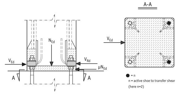
The design value of the shear force for a single column shoe on the active side, see Figure 6, is calculated from
