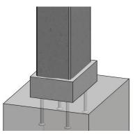
In column to foundation connections wider grouting can be provided to ensure higher concrete cover if it is required. It is recommended to increase the cover in aggressive environment.
