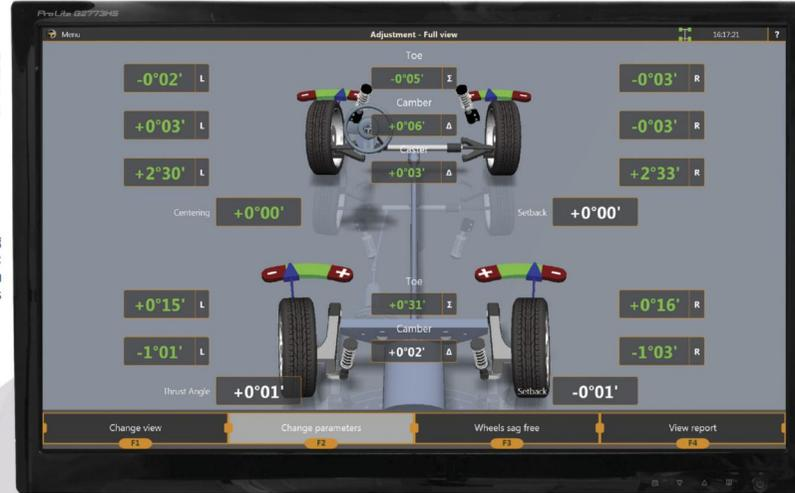
Measurements are automatically compared with standard specifications
