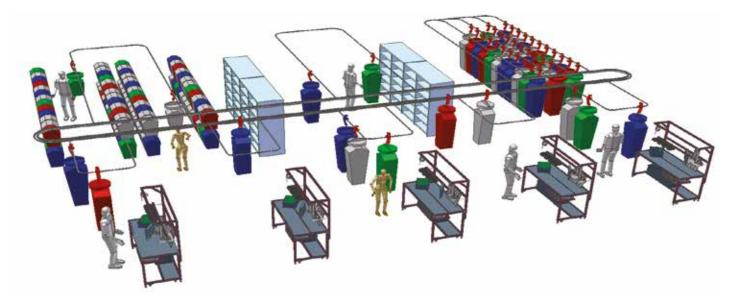
The conveyor line - is simple, reliable and almost silent. The drive mechanism consists of a rotating shaft that is powered by a worm gear motor. The travel speed may be varied from 1 to 30 m/min. It is possible to run sections of the conveyor at different speeds as well as backward and forward. Drives can be equipped with frequency converters giving very smooth start and stop movements in individual positions.
