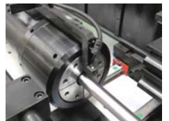
Welding detection There's also the option to add welding detection unit.
