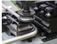
Multi-stack capability Ce CNC R models are available in single or multi-stack, fix and variable radius capability.
