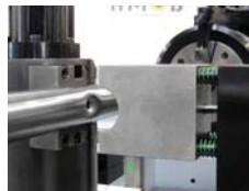
Punching unit On request, a punching unit can be added to the eMOB series.
