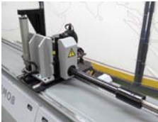
Servo controlled POB All Ce CNC R plane of bend positioners are servo controlled (up to 4 axis).
