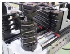
Multi-stack capability All eMOB models have multi-stack, fix and variable radius capability.
