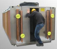
Opposite the control end is a large access door for entry into the coil air plenum. The door allows for visual in spection of the inner coil fins and acces to the fan motor if needed. Each cell can be separated by internal divider plates.
