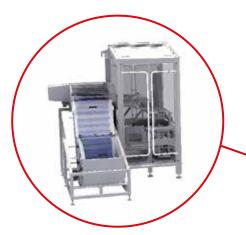
Module I: Infeed Module Infeed of the cups are done with a horizontal buffer as standard.
