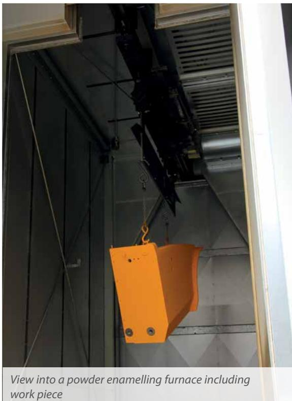
View into a powder enamelling furnace including work piece
