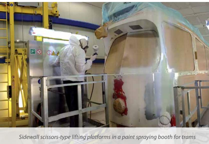
*Sidewall scissors-type lifting platforms in a paint spraying booth for trams*
