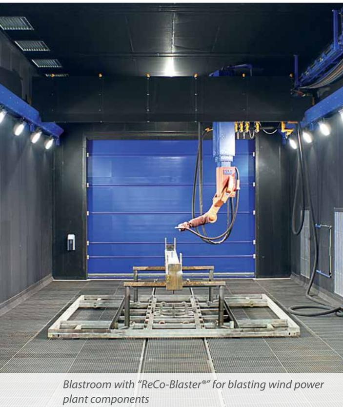
*Blastroom with "ReCo-Blaster®" for blasting wind power plant components*
