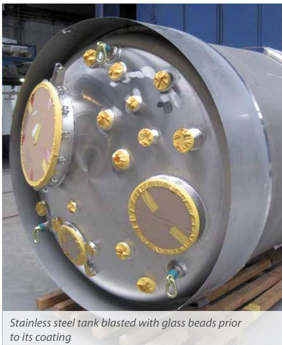
*Stainless steel tank blasted with glass beads prior to its coating*
