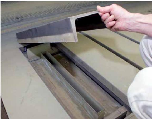
The heavy duty impact separators are the first step of our two stage paint separating system. Due to their special construction, heavy transport devices can drive on the impact separators without problems.
