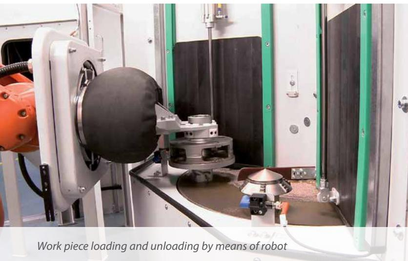
*Work piece loading and unloading by means of robot*
