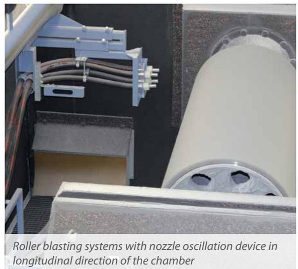
*Roller blasting systems with nozzle oscillation device in longitudinal direction of the chamber*
