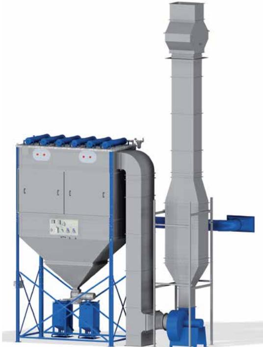
Zinc spraying (metallizing) is performed manually in special zinc spray booths, they consist of a zinc spray chamber, a movable suction hood for zinc overspray and a dust collector with limestone powder dosing and a CO<sub>2</sub> fire extinguishing unit. Such equipment for zinc spraying can also be retrofitted in existing blastrooms.
