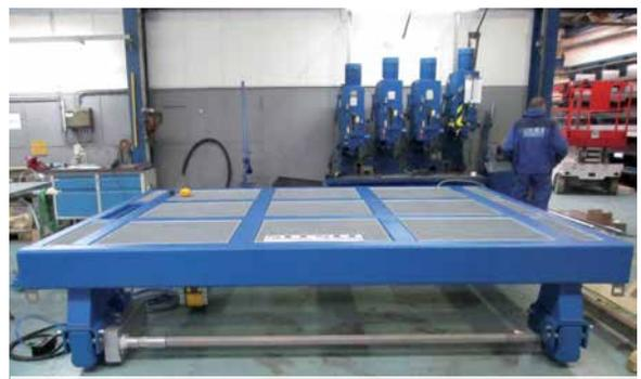
Electrically driven rail-bound trolley with lifting table
