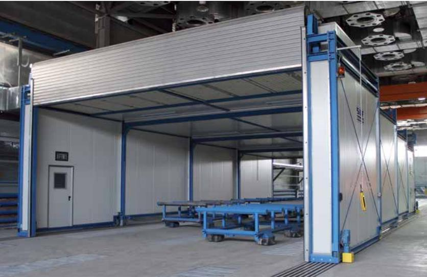
*Movable and telescopic dryer with open-space paint spraying system*
