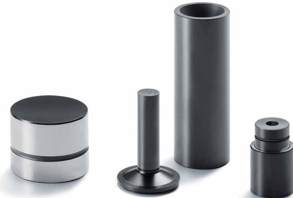
DLC coated piston pin used in bushing free aluminum pistons of gasoline and diesel engines to minimize wear and friction losses
