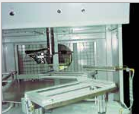
Standard ion luftkniv renser metalrammer inden pulverlakering.
